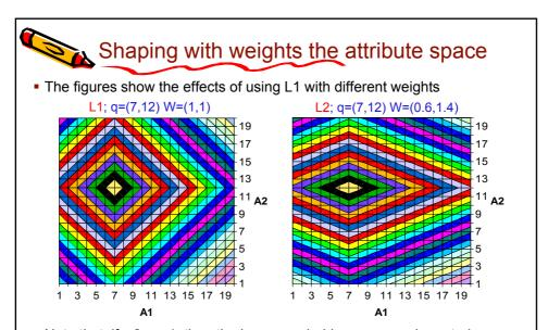
Note that, if w2 > w1, then the hyper-romboids are more elongated along A1 (i.e., difference on A1 values is less important than an equal difference on A2 values)
