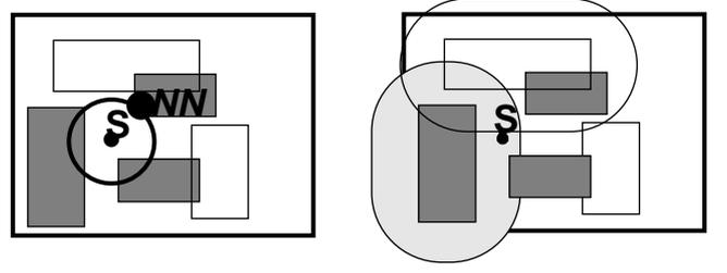
**Figure 3: Transforming a Spherical Query into a Point Query by the Concept of Minkowski Sum**
