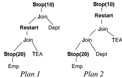
Figure 2: Aggressive Stop Push-Down for a 3-Way Join
