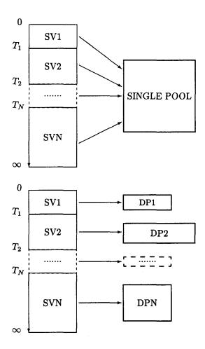
Fig. 1: Single-Pool and Multi-Pool Schema Versioning.
